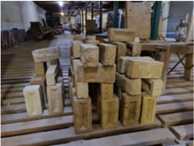
Patterns for stacking bricks in drying room
