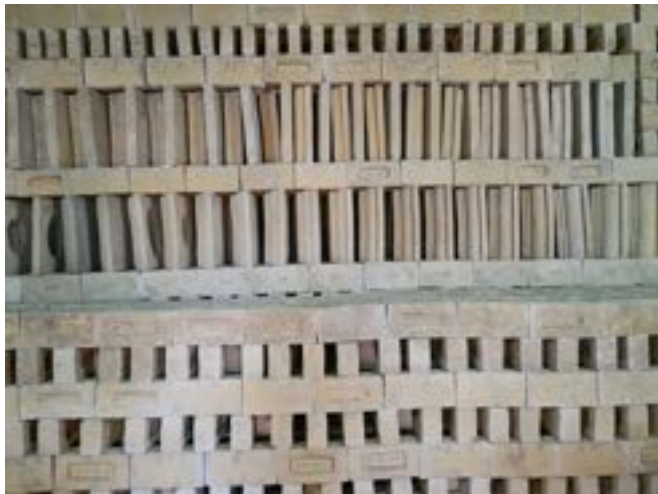
Patterns for stacking bricks in kiln
